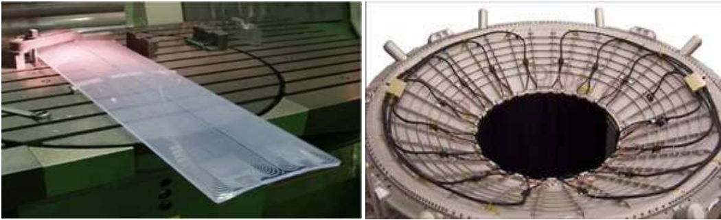
Figure 3.13: Left: ACC panel production Right: The Anti-Coincidence Counter integration in the Vacuum Case.
