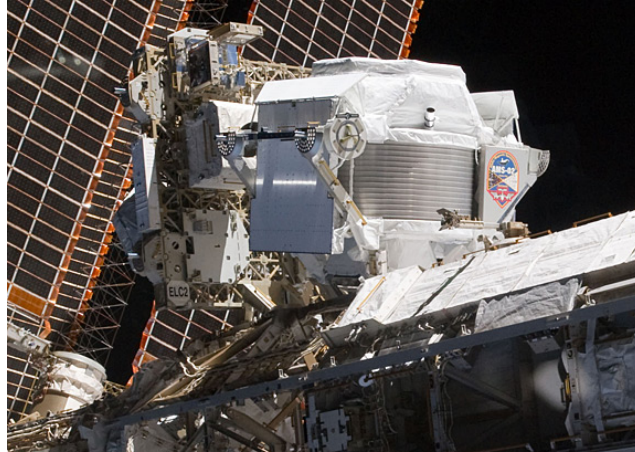
FIGURE 2.2: AMS-02 detector mounted on the upper Payload Attach Point on S3 Truss of the International Space Station.
